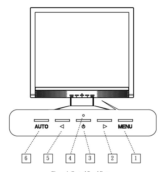
Figure.4. Control Panel Buttons
